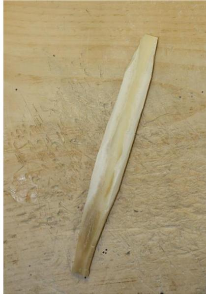
We chose from these fragments and tried to envision the tool that would emerge as we filed them into their final forms. The bones were then rough shaped with a hatchet, if needed. We began to refine the shape of the tools with farrier's rasps. We then worked through progressively finer files to shape the bone tools to fit our hand and suit our needs.
